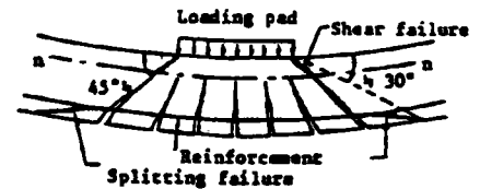
Fig. 2 Modeling of punching shear failure of slab.
