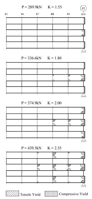
Fig.16 Progressive yield process of pipe
