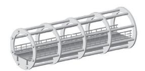
Fig.2 Tubular Bridge with steel pipes
