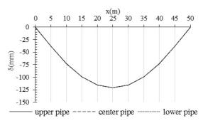
Fig.9 Vertical displacement of girders (D+L)
