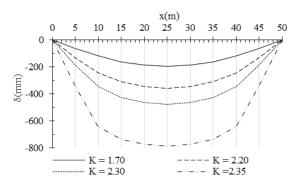
Fig.15 Vertical deflection of lower pipe girder
