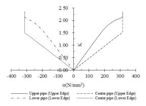
Fig.14 Stress vs. K of girders at R10
