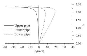
Fig.12 Longitudinal displacement at R10
