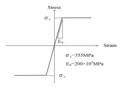
Fig.14 Stress vs. Strain of steel
