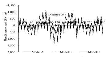
Fig.12 Bending moment of arch rib (D+L2)
