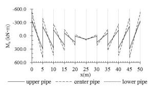
Fig.8 Bending moment of pipe girders (D+L)
