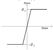
Fig. 10 stress vs. strain (SM490)
