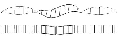
Fig.24 Side and top view of final deformation of Model A, 2.55 (D+L2)
