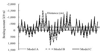
Fig. 10 Bending moment of girder (D+L2)
