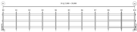
Fig.3 Side view of tubular bridge (unit: mm)
