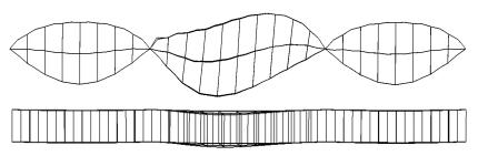
Fig.26 Side and top view of final deformation of Model C, 2.44 (D+L2)
