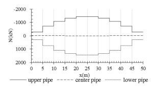
Fig.7 Axial force of pipe girders (D+L)
