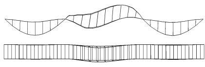
Fig.25 Side and top view of final deformation of Model B, 2.54 (D+L2)
